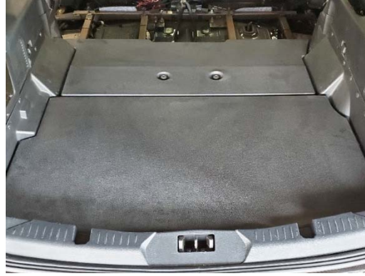
Remove rear floor sections. T-55 Torx socket will be needed for the forward floor section bolts.
