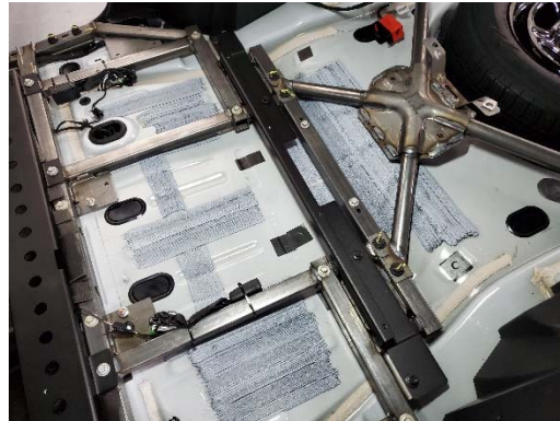
Use OEM bolts to attach K9 kit rear floor bracket to OEM cross brace.
