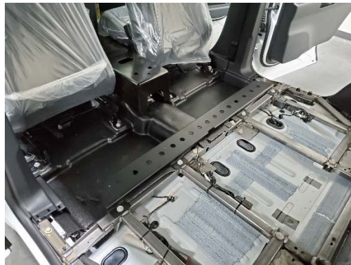
Use OEM bolts to attach K9 kit front floor bracket to OEM seat mount locations.
