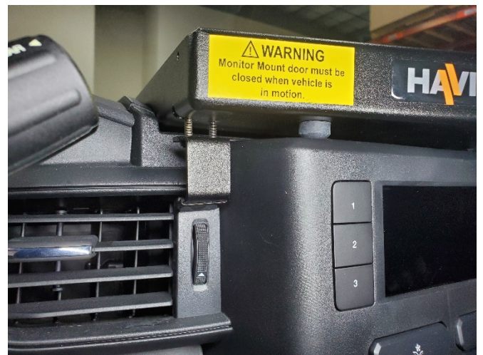
Place DMM tray onto upper dash and push towards the windshield. Lower mounting tabs should sit around trim by vents as shown.
