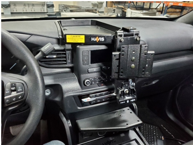
Test up and down motion of the arm and confirm smooth operation.
